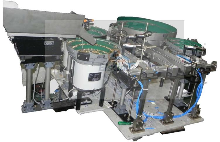
The other bowl was for caps to be fitted onto the container. The caps were having dia 30 mm x 10 mm thickness. Most of the caps came with the open end up. These were required to be fed with open end down. Hence, a sector type gravity track was designed for twisting them in 180 degrees. This was not attached to the bowl but mounted separately.
